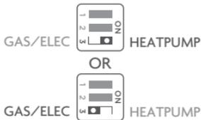
This dip switch configures the thermostat to control a conventional gas/electric system or a heat pump. If your system is anything other than a heat pump, leave this switch set for **GAS/ELEC**.
